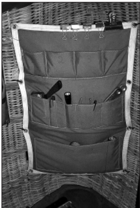
Cannon's self-styled basket organizer, a place for everything, everything in its place. The back side of the organizer can be built with an attached duffel to accommodate helmets and other bulky items.
